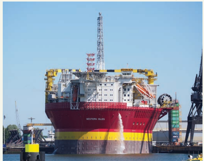
Floating production, storage and offloading vessels temporarily store oil at the offshore production site until it can be transported to shore by a barge or shuttle tanker.
